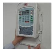
Secure the Indicator Station in place, using the pozi-drive machine screw provided.
